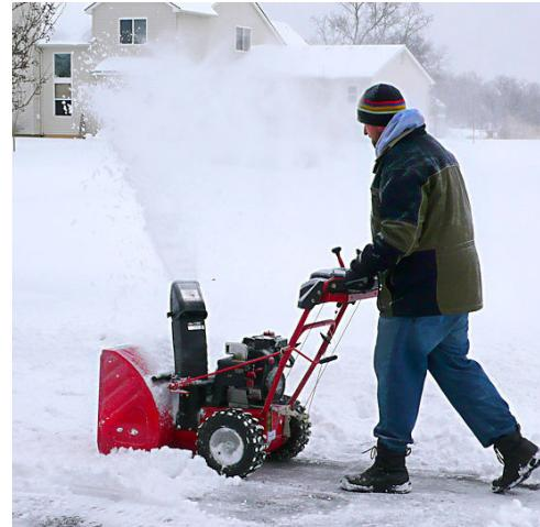
Always keep hands and feet away from all moving parts of the machine. Never place your hands in the auger. If the machine clogs while removing snow, shut the machine off and wait for all moving parts to stop. Some manufacturers recommend removing the spark plug wire from the spark plug. Remove snow with a stick or a similar instrument. Be prepared for a clogged machine to jump once the obstruction has been cleared.
